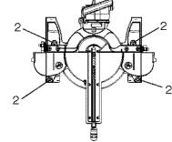
REMOVING AND INSTALLING THE TABLE INSERT (FIG. F)
